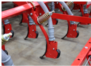
Heavy Duty Coil Sprung Tine with Unique Seed Boot
