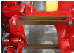
Unique Parallel Linkage for Contour Following
